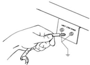
If you are not using a continuous or a constant monitor, a wrist strap should be tested while being worn at least daily. This quick check can determine that no break in the path-to-ground has occurred. Part of the path-to-ground is the perspiration layer on the person; an operator with dry skin may inhibit the removal of static charges and may cause a test failure.
