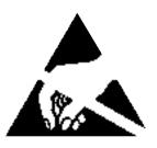
The ESD Sensitivity Symbol (also called Susceptibility or Warning Symbol) identifies items that can be damaged by ESD and should be unpackaged and handled while grounded at an ESD protected workstation.
