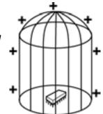
To complete the enclosure, make sure to place lids on boxes or containers, and close shielding bags. Packaging with holes, tears, or gaps should not be used as the contents may be able to extend outside the enclosure and lose their shielding as well as mechanical protection.
