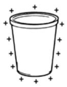
Insulators like this plastic cup will hold the charge and cannot be grounded and "conduct" the charge away.
